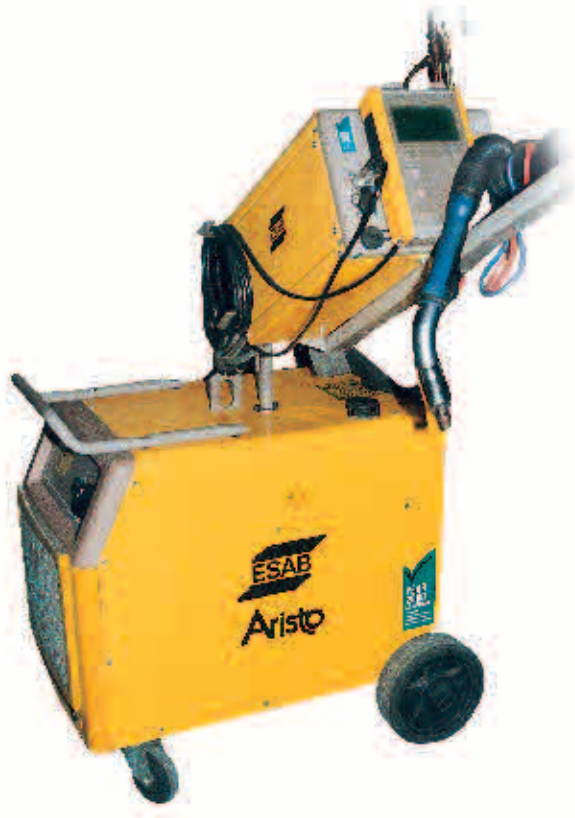
Figure 3. Multi-function welding unit Aristo 2000 LUD 450.
