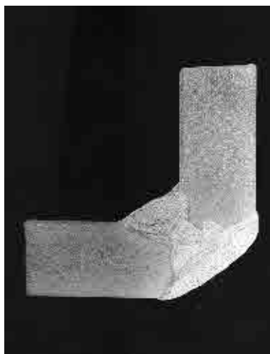
Figure 4. Cross-section cut through a corner seam welded with OK Autrod 18.16.
